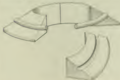
SECTION SHOWING STAGGERED CORNER OF FIELD MAGNET CORE
